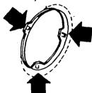
**4.** Reach through the rear exhaust opening and depress center of tabs on the plastic opening cover on the side you want to exhaust through. Remove the cover. Repeat for other dryer.
